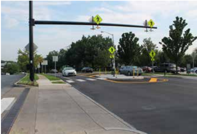
Rectangular rapid flashing beacons, a highly visible continental crosswalk, and a pedestrian refuge island with flexible delineators make this mid-block crosswalk on a high traffic volume roadway in Lower Merion Township safer for pedestrians.
